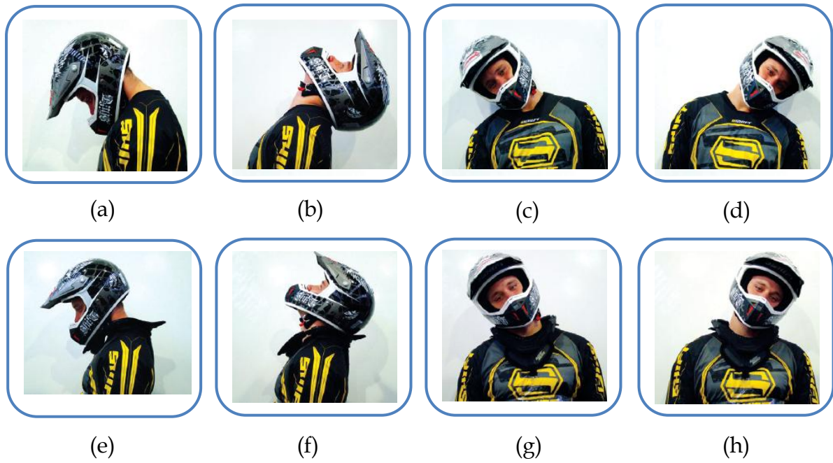
Figure 3-1: Extreme head movement without and with the Moto GPX
