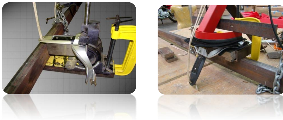
Figure 4-24: Test setup for thoracic strut bending moment
