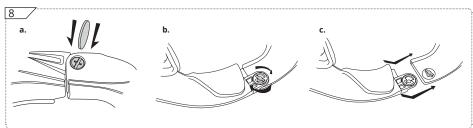
The emergency open is used when the whole front of the brace needs to be removed. Any object with a flat solid surface can be used to turn the emergency open screw. After the screw has been turned the brace can be opened from the left side as well.
