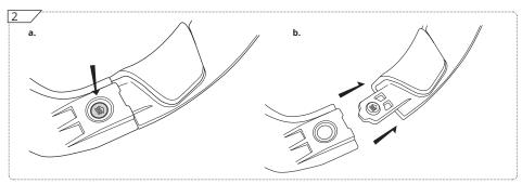
Open the brace by pushing the release button underneath the right side of the brace (2a). You can now pull the brace open (2b).
