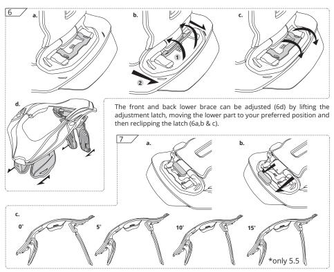
If you feel the brace "climbing" your back, adjust the rear thoracic by swopping the rear thoracic angle wedges around (7a & b). The wedges are easily interchangable and their are four kinds of wedges for different body types (7c).
