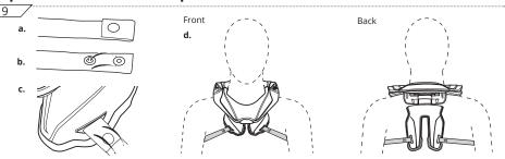
The brace strap is easily attached through opening the ends of the straps (9 a & b), looping them through the strap openings and then closing them again (9.c & d). Please make sure you have the straps secure on the front and back of the brace(9.e).
