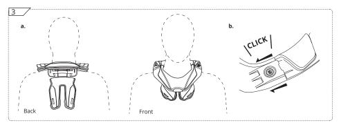
Fit the brace with the rear thoracic facing your back (3a). Close the brace, there should be a click to confirm that it is closed (3b).
