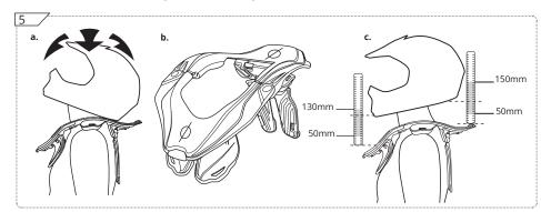
Check that you have the right helmet rim clearance. Please use assistance to do this measurement, do not do it yourself. Place a ruler in the middle of the upper rim of the brace at 90<sup>0</sup> to the ground, with your head in a neutral (level) position (5b). Remember to do front and back. The helmet rim should be within the zone of optimum effectiveness (5c)
