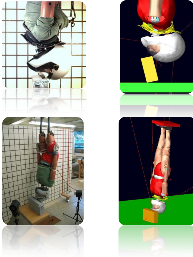
Figure 4-2: Pendulum test and simulation setup
