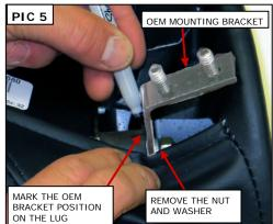
Refer to PIC 5. Remove the nut and lock washer securing the mounting bracket to the rubber lug. Remove the OEM bracket and set it aside; it will not be re-used.
