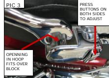
STEP 4 With the legs of the hoop over the blocks in the mounting brackets, rotate the Backrest assembly towards the back of the motorcycle until it is in the upright position. PIC 4
