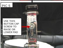
To raise or lower the Backrest pad, fold the pad up and slightly loosen the button cap screw on the post. PIC 5 Raise or lower the pad to the desired position, (there are detents inside the post that attaches the pad to the hoop that you may feel or here click as you move the pad). Tighten the button cap screw securely to lock the pad in place if you would like to maintain one set position.
