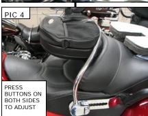
To move the Backrest assembly forward or backward, push and hold the release buttons on each of the mounting brackets and slide the assembly along the track. Once the desired position is found, release the buttons. With the buttons released, ensure that the Backrest assembly has locked into place. PIC 3 and PIC 4
