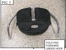
STEP 8 To store the Backrest assembly in the trunk of the motorcycle, tip the assembly forward and remove it from the mounts. Fold the Backrest pad forward until it is beneath the hoop. The assembly will now fit in the trunk. PIC 7 and PIC 8
