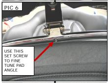
To fine tune the angle of the Backrest pad, turn the set screw on the underside of the hoop in to tilt the pad forward or out to tilt it back to the upright position. PIC 6
