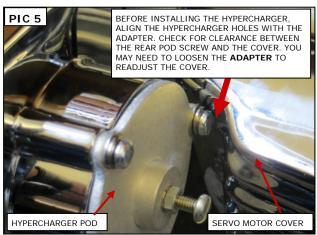
ALIGN THE HOLES AND APPLY GASKET
