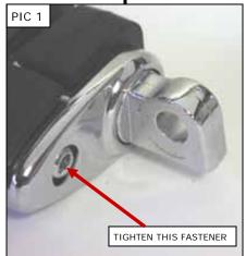
FOOTPEGS MUST BE INSTALLED SO THEY WILL FOLD UPWARD AND REARWARD IF HIT BY ANY OBJECT. FAILURE TO ADJUST THE FOOTPEGS TO OPERATE IN THIS MANNER COULD RESULT IN SERIOUS INJURY OR DEATH.
