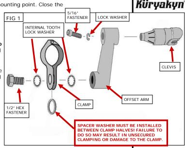
STEP 5 The angle of the clevis may be adjusted by loosening the 5/16" fastener that secures the clevis to the arm. FIG 1 Rotate the clevis and peg to the desired position. Tighten the fastener securely.
