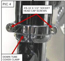
When installing the neck covers, you will need to slightly push down while tightening the top fastener. This will allow adequate clearance between the top of the neck covers and the inner fairing or headlight shroud when the bars are rotated all the way side to side.
