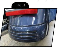
**STEP 5** Rub the adhesive backing on the accents to activate the adhesive. Remove the tape backing and apply the accents to the lower fender one at a time.
