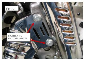
**STEP 4** Check the bottom of the caliper cover to make sure you have clearance from the brake rotor and tire valve stem. PIC 3
