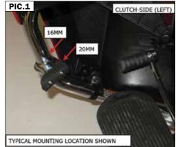
**STEP 6** Ensure that the position of the Toe Rest does not interfere with the proper operation of the motorcycle **BEFORE** riding.
