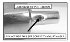
STEP 8 Refer to PIC 4. Install the included set screws in the lower holes on the Tour Tech™ arms. Turn the set screws in or out to adjust the angle of the footrest.
