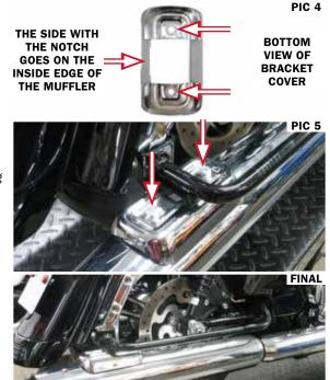
**STEP 6** Refer to PIC 5. Install the covers over the muffler brackets.
