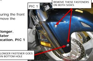
STEP 3 Remove the stock chrome fork cover. Remove the two front screws (PIC 2) and dislodge the plastic
