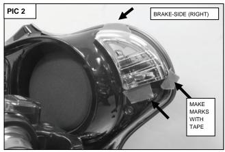
NOTE: If the bike is going to be operated before full bonding occurs, secure the Accent to the fairing with a good
