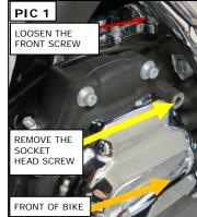
STEP 3 Remove the transmission bearing housing screw shown in PIC 1 on PAGE 1; place one of the included Spacers over the screw as shown in PIC 2; set it within arms reach of the work area.
