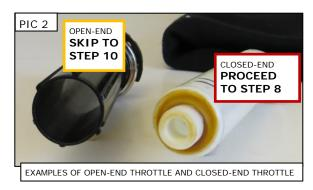
ONLY FOLLOW THE INSTALLATION INSTRUCTIONS FOR YOUR TYPE OF THROTTLE SLEEVE. FAILURE TO DO SO COULD RESULT IN DAMAGE TO THE GRIP, THROTTLE SLEEVE OR HANDLEBAR.
