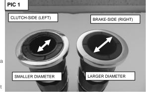
**STEP 5** Locate the throttle-side Grip; it has a slightly larger inside diameter than the clutch-side Grip. Decide if you want the throttle-side Grip's pads to match the clutch side when the bike is at rest or underway with the throttle slightly opened. Without using the included glue, slide the Grip into place and determine its position. Mark the positions of both Grips and switch housings with a non-permanent marker. Remove the Grips.
