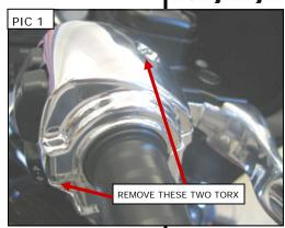
STEP 5 Re-assemble the switch housing halves and secure them with the screws removed in Step 2. Ensure that the end of the throttle grip locates in the channel in the switch housing. Tighten the brake clamp if it was loosened in Step 2.
