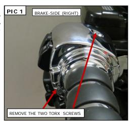
STEP 3 Gently separate the housing halves and slide the existing grip off of the handlebars. Set it aside, it will not be re-used.
