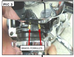
**STEP 10** Adjust the throttle cables and tighten the jam nuts. Ensure proper throttle cable adjustment and throttle operation before riding the motorcycle. Refer to your model owners' manual or service manual for more information.
