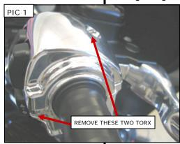
STEP 5 Reassemble the switch housings using the two Torx screws that were removed in STEP 2. Tighten the screws on the brake clamp if they were loosened.
