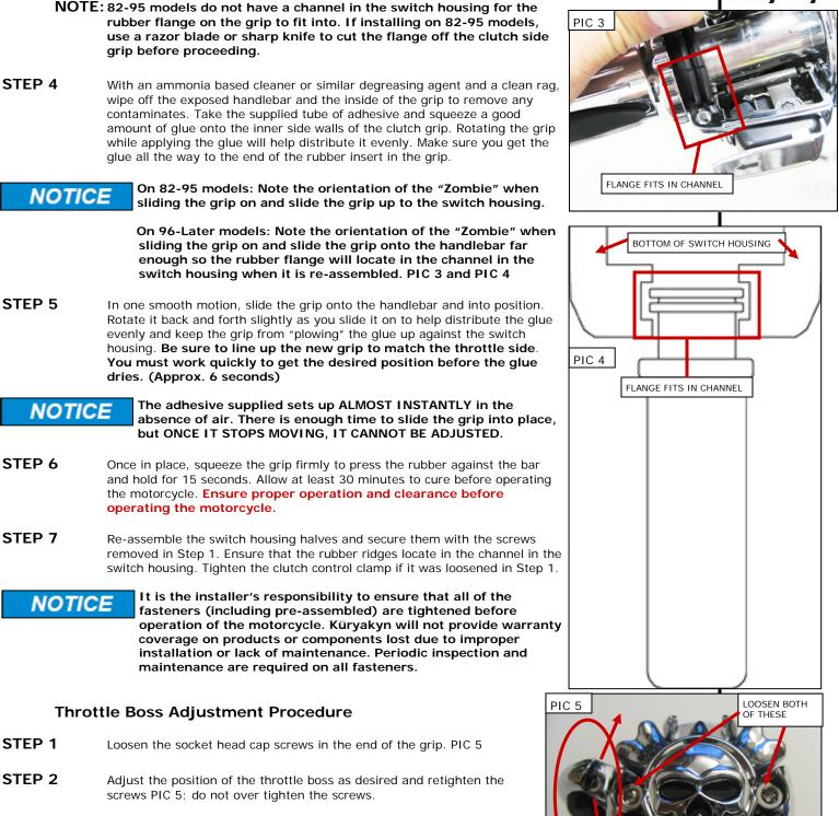
**NOTICE** It is the installer's responsibility to ensure that all of the fasteners (including pre-assembled) are tightened before operation of the motorcycle. Küryakyn will not provide warranty coverage on products or components lost due to improper installation or lack of maintenance. Periodic inspection and maintenance are required on all fasteners.
