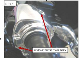
ROTATE THROTTLE AND CHECK THAT IT MOVES FREELY AND RETURNS WARNING TO CLOSED BEFORE STARTING BIKE. FAILURE OF THE THROTTLE TO PROPERLY RETURN COULD RESULT IN LOSS OF CONTROL CAUSING SERIOUS INJURY OR DEATH.
