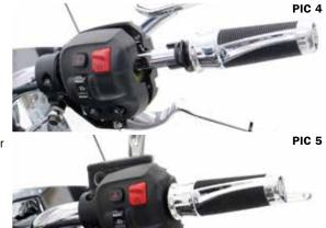
STEP 6 Refer to PIC 5. Reassemble the switch housing and secure with the four (4)screws that were removed in Step 3. Reassemble the brake lever/master cylinder assembly onto the handlebar.
