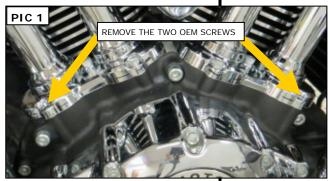
**STEP 5** Torque the screws to 85-115 in lbs (9.6-12.9 Nm).
