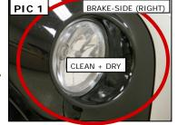
**STEP 3** Refer to **PIC 2**. Determine the Left and Right Driving Light Bezel. The notch is in the topside. PIC 2 NOTCH TOWARDS TOP BRAKE-SIDE (RIGHT) CLUTCH-SIDE (LEFT)
