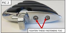
FOOTPEGS MUST BE INSTALLED SO THEY WILL FOLD WARNING UPWARD AND REARWARD IF HIT BY ANY OBJECT. FAILURE TO ADJUST THE FOOTPEGS TO OPERATE IN THIS MANNER COULD RESULT IN SERIOUS INJURY OR DEATH.
