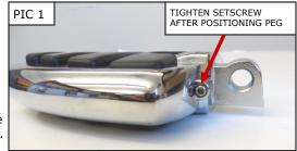
STEP 3 Install the new peg using any spacers or washers removed in Step 2. Line up the hole on the male mount on the new peg with the hole in the clevis.
