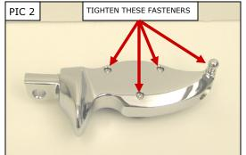
STEP 5 Secure the peg in the clevis using the OEM hardware removed in Step 3. Check that the peg is installed correctly and is able to fold upward.
