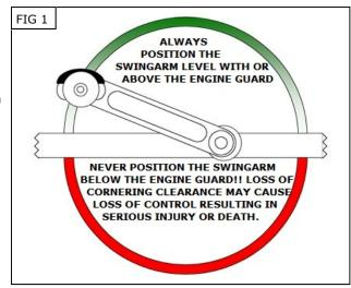
WARNING IT IS THE INSTALLERS RESPONSIBILITY TO ENSURE THERE IS SUFFICIENT CORNERING CLEARANCE BEFORE RIDING. ALWAYS POSITION THE MINI ARM EITHER LEVEL WITH, OR ABOVE THE ENGINE GUARD. POSITIONING
