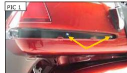
STEP 3 "Drop" the rear portion of the bottom panel of the trunk. The bottom panel is secured by three Phillips head screws across the back; under the center molding you just removed. There are also
