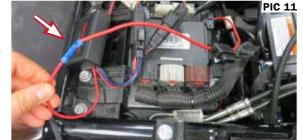
**STEP 11** Refer to PIC 11. Locate the single RED wire from the Relay Module.
