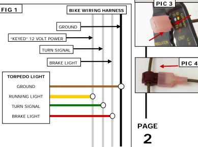
TORPEDO LIGHTS with RUN-TURN-BRAKE FUNCTION
