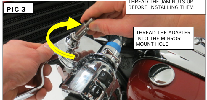
PIC 2 THREAD THE JAM NUTS UP BEFORE INSTALLING THEM
