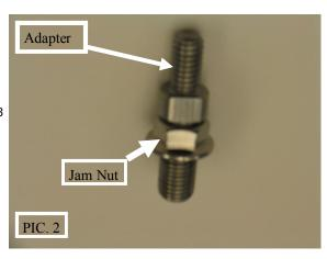
**STEP 6** Holding the adapter with a wrench in adjusted position, tighten jam nut to the stock mirror mounting point.
