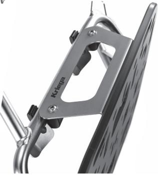
**3.** Fit the remaining 4 x alloy clamps in the positions as illustrated below. Once all clamps are in place and the OS-Platform is level with the frame you can fully tighten all the bolts.
