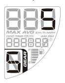
The main screen now displays the number 5, slow down and wait until the meter goes back to the main screen.
