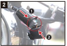
2. plug the connector in with the vehicle main harness connector. The pull back the waterproof cover to fully cover the both connectors & vehicle main harness connector). NOTE waterproof cover from KOSO BOLT Meter needs to be overlapped with vehicle main harness rubber connector cover.
