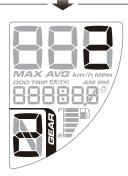
When the number 2 is flashing, put the motorcycle in 2nd gear and start riding slowly until the meter detect the correct gear. Once the meter has detected the 2nd gear, the screen will automatically switch to number 3.
