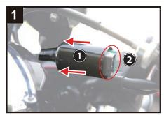
1.Push the waterproof cover of the KOSO BOLT Meter **1** until the connector **2** is exposed outside the cover.
