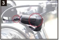
3.Wrap up insulation tape on waterproof cover, wiring PVC pipe and the gap between the waterproof cover and original waterproof cover,as shown in the red circled part.
