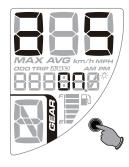
In gear learning screen, press and hold the SELECT button for 3 seconds to enter settings screen.
