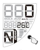
$\bullet \mbox{In}$  the temperature screen, press the  $\mbox{\bf SELECT}$ button once to switch to the voltage screen.
