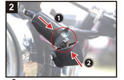
2. plug the connector in with the vehicle main harness connector. The pull back the waterproof cover to fully cover the both connectors & vehicle main harness connector).
