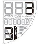
When the number 3 is flashing, put the motorcycle in 3rd gear and start riding slowly until the meter detects the correct gear. Once the meter has detected 3rd gear, the screen will automatically switch to number 4.
