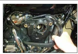
6. Remove the air filter base from the vehicle as shown.
