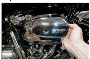
2. Remove air filter cover bolt and air filter cover as shown.
