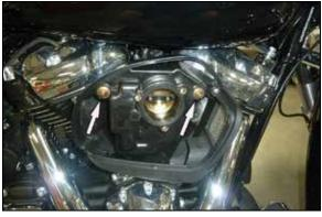
5. Remove the two breather/air filter base mounting bolts as shown.
