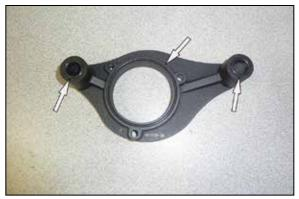
7. Install three of the O rings provided onto the back side of the K&N® back plate as shown.
