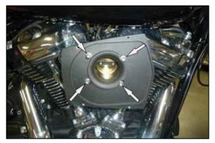
10. Install the air scoop base gasket and base plate with the provided hardware. Slightly tighten at this time. Using the air filter cover clock the filter base in position then finish tightening filter base plate.
