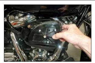
4. Remove the air filter from the vehicle and disconnect the crankcase breather tubes.
