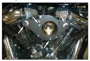
9. Using the two provided crankcase breather bolts; install the back plate onto the vehicle. Do not tighten bolts at this time. Make sure O rings do not fall out during this operation. Install the two allen bolts and tighten all bolts at this time.
