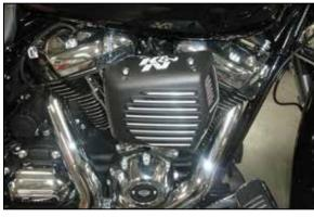
11. Install the  $K\&N^{\otimes}$  air filter and filter cover with provided bolts.
