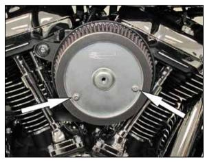
13. Install the filter onto the back plate and secure with the provided hardware.
