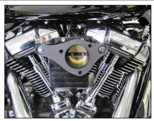
8. Using the provided throttle body mounting bolts, install the base plate onto the engine. Do not completely tighten the bolts; they are just being used to hold the base plate in the correct position at this time. Secure the servo cover to the back of the base plate with the hardware provided. Now install the remaining breather O-rings into the base plate and secure the base plate with the provided breather bolts. Then remove the three throttle body bolts.
