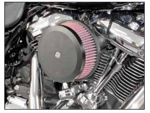
14. Install the top plate onto the filter and secure with the provided hardware. **NOTE: Apply one drop of the provided thread**
