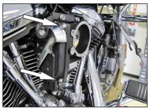
5. Remove the two servo cover bolts shown.
