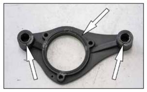
7. Install two of the breather O-rings and the throttle body O-ring into the base plate as shown. **NOTE: Use a few small dabs of grease to secure the O-rings in place while installing the base plate to the engine.**
