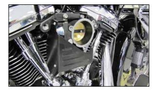
2. Loosen and remove the bolt which secures the decorative filter cover and remove the cover from the vehicle.
