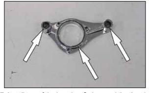
7. Install two of the breather O-rings and the throttle body O-ring into the base plate as shown.
