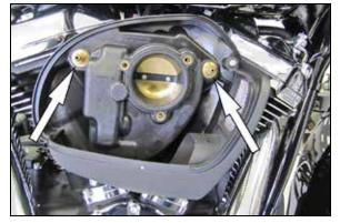
4. Remove the two breather bolts shown and then remove the rear air filter housing from the vehicle. NOTE: K&N Engineering, Inc. recommends that customers do not discard the factory air intake components..
