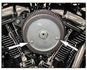
13. Install the filter onto the back plate and secure with the provided hardware.
