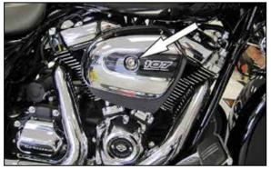
2. Loosen and remove the bolt which secures the decorative filter cover and remove the cover from the vehicle.
