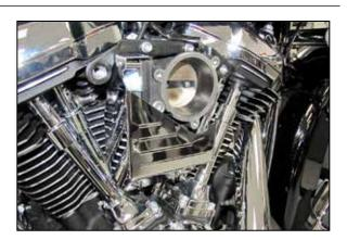
6. Install the K&N® servo cover and secure with the provided hardware to the original servo cover mounting bolt locations.
