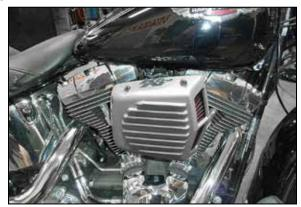
13. Install air filter and air filter cover with provided bolts.
