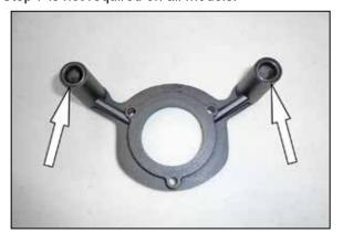
8. Install two o rings provided onto the back side of the  $K\&N^{@}$  back plate as shown.
