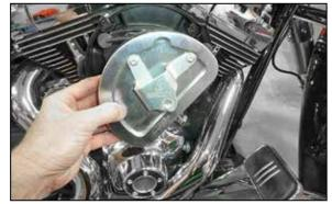
4. Remove the air filter with breather hoses as shown.
