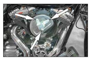
3. Remove the three air filter retaining bolts as
