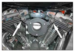
10. Using the two provided crankcase breather bolts install the back plate onto the vehicle as shown. Do not tighten the breather bolts at this
