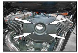
12. Install the provided gasket between the back plate and air filter base using provided hardware. Slightly tighten at this time. Using the air filter cover clock the filter base in position then finish tightening filter base plate.
