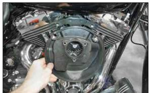
6. Remove the air filter breather base as shown. NOTE: K&N Engineering, Inc. recommends that customers do not discard the factory air intake components.
