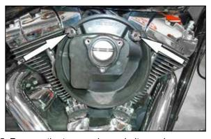
5. Remove the two crankcase bolts as shown.
