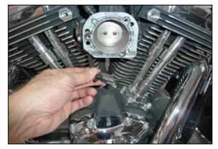
7. Using the provided tie wrap, secure the loose pigtail to the throttle position switch wiring harness. Step 7 is not required on all models.
