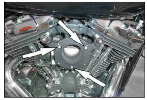
11. Install the provided gasket between the throttle body and back plate use the provided hardware to secure the back plate to the throttle housing. Tighten the crankcase breather bolts.
