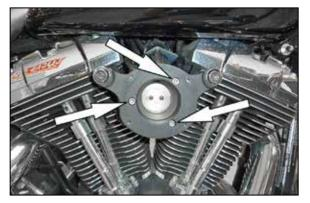
10. Install the provided gasket between the throttle body and back plate use the provided hardware to secure the back plate to the throttle housing. Tighten the crankcase breather bolts. **NOTE: Apply one drop of the provided thread locker onto the provided bolts.**
