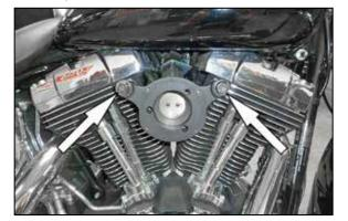
9. Using the two provided crankcase breather bolts install the back plate onto the vehicle as shown. Do not tighten the breather bolts at this time. **NOTE: On applications that have had the support bracket removed, install the two provided spacers between the back plate and cylinder head at the breather holes and then install the breather bolts as shown.**
