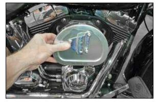
4. Remove the air filter with breather hoses as shown.
