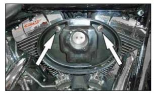
2. Remove the air filter cover retaining bolt and then remove air filter cover as shown.
