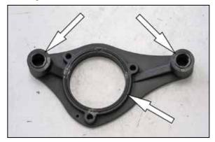
7. Install two of the breather O-rings and the throttle body O-ring into the base plate as shown. NOTE: Use a few small dabs of grease to secure the O-rings in place while installing the base plate to the engine.
