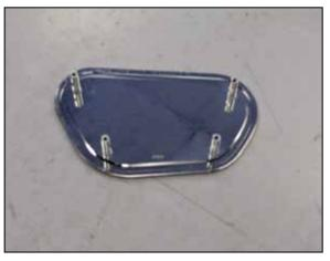
11. Install the four provided spacer bolts and washers into the filter top plate as shown.
