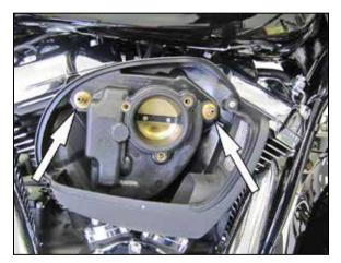
4. Remove the two breather bolts shown and then remove the rear air filter housing from the vehicle. NOTE: K&N Engineering, Inc. recommends that customers do not discard the factory air intake components.
