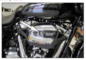
2. Loosen and remove the bolt which secures the decorative filter cover and remove the cover from the vehicle.
