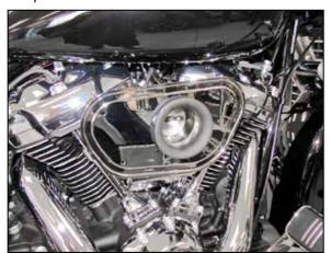
10. Using the three provided throttle body bolts, secure the filter back plate to the base plate as shown.
