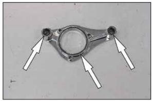
7. Install two of the breather O-rings and the throttle body O-ring into the base plate as shown.
