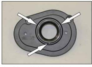
5. Install the provided venturi and the three throttle body mounting bolts into the back plate as shown. NOTE: The bolts pass through the back plate and venturi on the back side.
