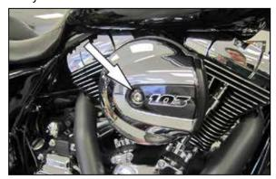
2. Remove the bolt which secures the bonnet to the filter assembly and then remove the bonnet from the vehicle.
