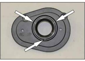
5. Install the provided venturi and the three throttle body mounting bolts into the back plate as shown. NOTE: The bolts pass through the back plate and venturi on the back side.
