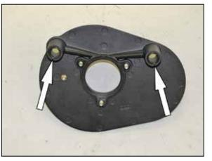
7. Install two of the provided O-rings into the crank case breather plate as shown.
