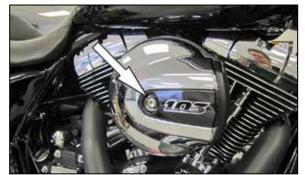
2. Remove the bolt which secures the bonnet to the filter assembly and then remove the bonnet from
