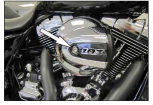
2. Remove the bolt which secures the bonnet to the filter assembly and then remove the bonnet from the vehicle.
