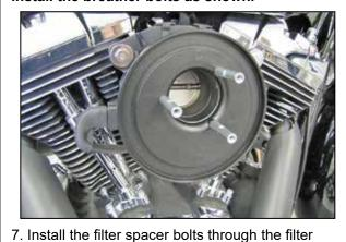
back plate and then install the gasket onto the spacer bolts passed through the back plate. Install the filter back plate assembly onto the breather plate and secure with the filter spacer bolts.
